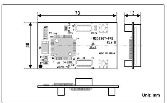
Figure 5.1 External dimensions of the M30220TF-PRB
